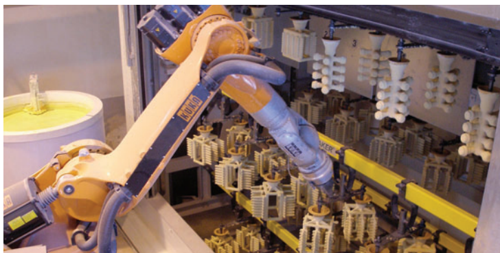
Robot and drying chamber for investment cast components. Excellent mould design allows for ideal structural conditions and outstanding wear resistance of components.
